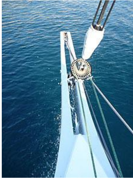
Water jet along the chain on the bowsprit. The bobstay is detachable
