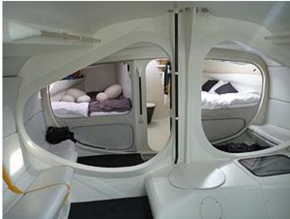
The interior of the JP54 looking forward. Look at the beautiful shape and flared openings of the central carbon bulkhead
