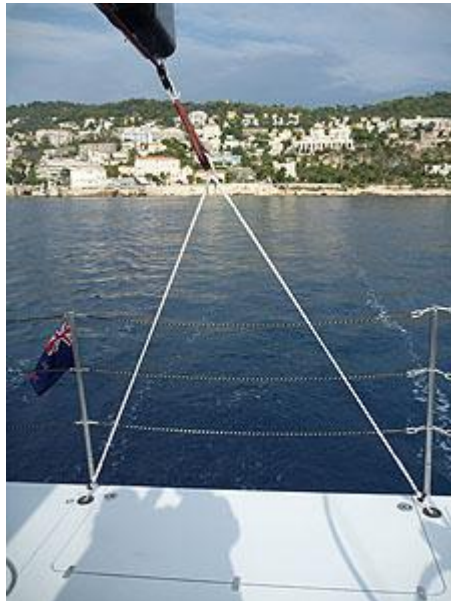
The mainsheet can be easily detached from these Spectra lines on dogbone fittings (below)
